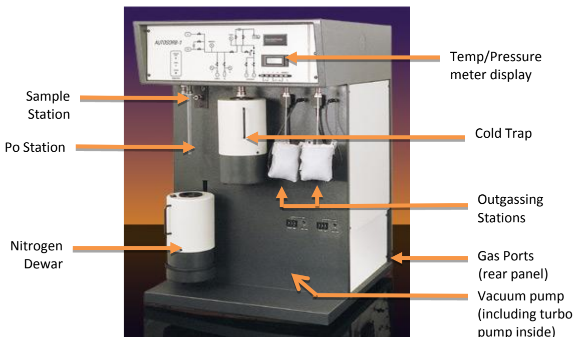
Figure 1.5. Image of Autosorb-1C with essential components labeled.
